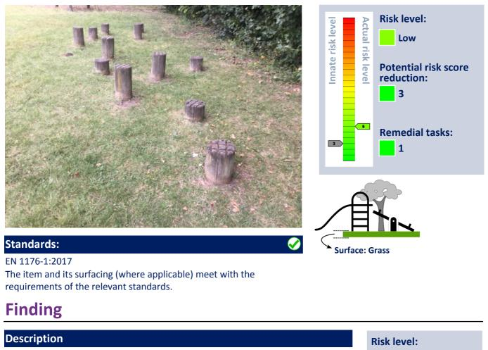
Strimmer damage to supports is likely to accelerate timber rot.
